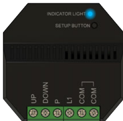
Blue flashing Indicator Light Network Pairing Mode
