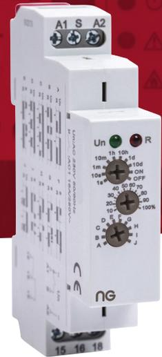
**Din rail mounting process timer in a din style housing. Multivoltage. 10 function. 16A changeover contact. LED indication for coil power and timer running.**
