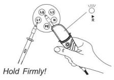
► L LED indicates that the field is rotating towards the left direction of the "probe -". With this connection, the motor will go negative rotation.
