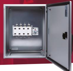
1250A 4 pole manual changeover switch in a metal enclosure to IP65. Enclosure has separate lock. The switch handle is padlockable and defeatable. Earth studs are fitted and fixing brackets and earth straps are included
