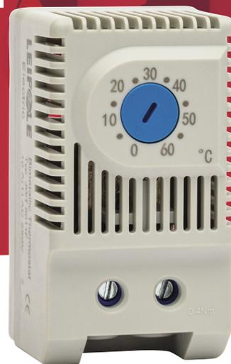
**Thermostat with a normally open contact, for use when the temperature exceeds the set value. Blue coloured control dial. Din rail mounting**
