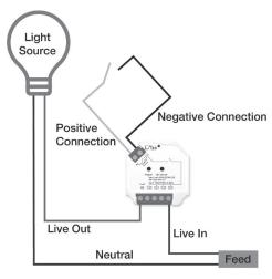
\*This option should be used with 1 switch only. For 2 way switching follow mains option
