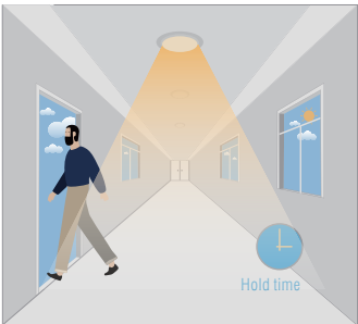
The sensor keeps light ON for holdtime period after motion leaves.
