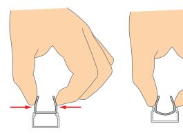
When inserting U-Clip 30 in 25x16mm trunkings, gently squeezing the upright tabs causes the base to compress for tight fitment in Size 2 trunkings.
