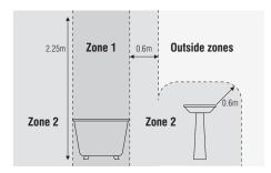
This product has no special protection against the ingress of moisture, and is rated as IP20. This product is suitable for use in outside Zones of a bathroom only. See diagram.
