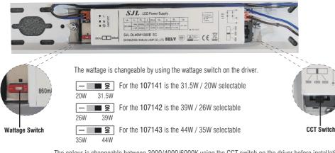
The colour is changeable between 3000/4000/6000K using the CCT switch on the driver before installation. Choose your preferred wattage and colour before installing by wattage switch or CCT switch on the driver. Note: Befeore you change the wattage or colour, please turn off the power switch for safety.
