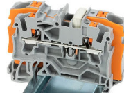
Step-down jumper (2006-499) commons 6/4 mm 2 (10/12 AWG) terminal blocks (2206/2204 Series) with 4/2.5/1.5 mm 2 (AWG 12/14/16) terminal blocks (2204/2202/2201 Series).
