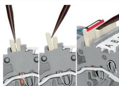
3- and 4-conductor terminal blocks (angled type): WAGO's TOPJOB® S Rail-Mount Terminal Blocks have a 35-degree conductor entry angle permitting a very small bend radius and an extremely short wiring distance to the cable duct. These are space- and cost-saving solutions for switchgear and control cabinet applications that use the LSC wiring system from Lütze. The design allows cable duct to be placed very close to the terminal blocks, keeping its height relatively low.
