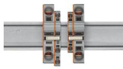
Stepping down via push-in type jumper bar: Commoning via open terminal side with end plate allows jumpering over two cross-section sizes for 16 mm<sup>2</sup> (6 AWG) and 10 mm<sup>2</sup> (8 AWG) and one cross-section size for 6/4/2.5 mm<sup>2</sup> (10/12/14 AWG). An example: from 16 mm<sup>2</sup> (6 AWG) to 6 mm<sup>2</sup> (10 AWG) (see illustration above) or from 10 mm<sup>2</sup> (8 AWG) to 4 mm<sup>2</sup> (12 AWG).
