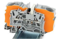
Step-down jumpers common terminal blocks of different sizes, without losing a conductor clamping point. This can be beneficial on long conductor runs where voltage drop can be a problem. A large conductor can be easily connected to smaller conductors at the distribution point. Commoning may be made in either direction using the special thin end plate to cover the open side. Additional through terminal blocks having a smaller cross-section may be commoned using push-in type jumper bars.
