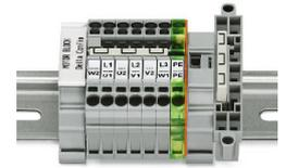
Continuous jumpers (2002 Series) readily connect an endless number of terminal blocks to each other via single jumper slot. Use the second jumper slot for additional commoning or testing.
