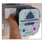
test. The LEDs will show all green with a continuous tone if the wiring is correct. Any other LED colour or warble tone indicates incorrect wiring and all further tests are inhibited. Check the indication displayed by the
