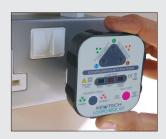
Flashing red LED with warbling means the earth path is over  $93\Omega$ . This may not be dangerous but the value should be checked using an earth loop tester with a read out to check the value meets the wiring regulations.
