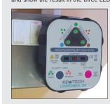
Green LED with continuous tone indicates the wiring condition is good with safety earth path less than  $1.80\Omega$ .
