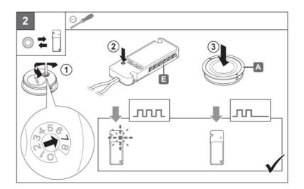
Pairing the Wireless Remote to the Receiver Module:
