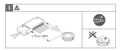
• Multiple Wireless Remotes (hand held remotes [833.89.121] and remote switches [833.89.122]) can be paired to each Receiver Module.
