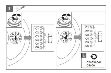
Test the pairing by pressing the power button <sup>(a)</sup> for on and off. [Turning the dial to 0 for all zones or individual zones (C1, C2, C3... 1, 2, 3...) (Dial position 1 = C1 etc., Dial position 0 = all zones)]. Note: C1 will turn all C1 lights on /off etc.
