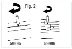
The wattage is changeable between **18W/24W** using the wattage switch for 59995. For the 59996, It is the 2- roots combination, there are **two18W/24W** selectable, Please put the adjusting switch on the same gear.
