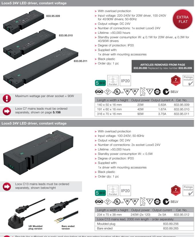
> Provide for sufficient air supply and circulation at the mounting location of the driver; we recommend 10 mm clearance Maximum lead length from the Loox5 driver to the light is 10 m. Long cable lengths in combination with large loads (strip light lengths) can result in voltage losses in the cable. These lead to visible loss of brightness in the lights. The illuminance listed with the lights has been determined with the rated output voltage of the driver (12V or 24V).
