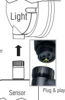
How to return to automatic sensor mode: Switch off the wall switch, wait 10 seconds and then switch it back on, then the sensor will be back in automatic sensor mode.
