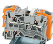
Step-down jumper (2006-499) commones 6/4 mm² (10/12 AWG) terminal blocks (2206/2204 Series) with 4/2.5/1.5 mm² (AWG 12/14/16) terminal blocks (2204/2202/2201 Series).
