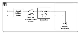
Alternatively they can be controlled by an independent controller that provides power on demand.
