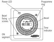
**Time control segments:** 1 segment = 15 minutes, push segment down for ON, pull up for OFF.
