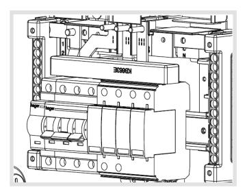
Clip the 4 module surge protection device to the dinrail next to the chosen incomer. (If 3 pole substitute the neutral connection block with the KRN199, copper neutral link and M6 carp nut and tighten the nut to 5Nm.
