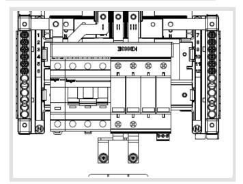
Place the copper earth component into the bottom two cage terminals and secure to 3.5Nm. Connect the opposite end to the enclosure using the 2 hex head high-tourge screws to 3.5Nm. and fit the shroud provided with the incomer kit by cutting out the extra modules to accommodate the surge protection device.
