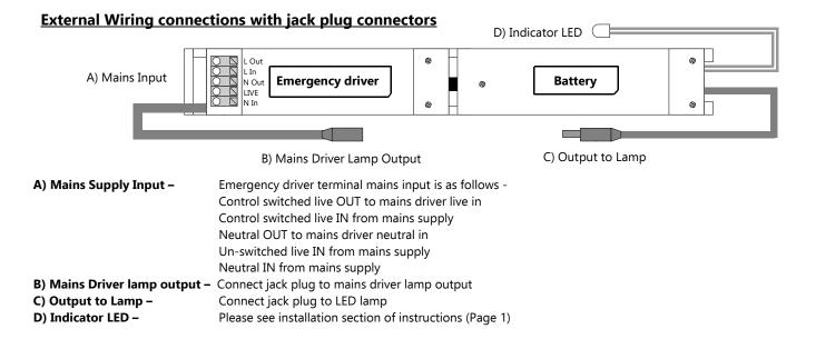
Note: Jack plug connectors appearance may change however connections will always be as follows: Mains driver lamp output from emergency driver side of enclosure. Output to lamp from battery side of enclosure.
