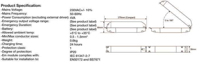
The unit provides reinforced insulation between the mains supply and battery charging circuit and employs self-resetting protection against short-circuit of battery terminals. Normal charging will resume automatically once a fault is removed.
