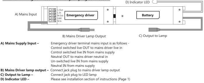
Note: Jack plug connectors appearance may change however connections will always be as follows: Mains driver lamp output from emergency driver side of enclosure. Output to lamp from battery side of enclosure.
