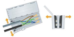
7. Try to keep cables of a similar size together in the same slot and simply **push them into the slot as** far as they will go. Once all the cables are installed, firmly squeeze the gripper end of the box together and snap shut the lid so that it is held securely by the 3 locking tabs.
