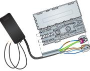
When fitting the cables into the cable clamp the sides of the box need to be eased apart to make an opening. It is normal for the entrance to be splayed apart with the cables in place.
