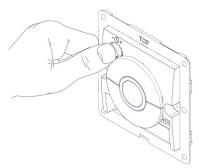
Time setting (determined by switch, see below) 5 sec—15min 15min—2hour
