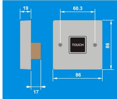
The ELLIPSE and KH2 time lag switches are a quick and effective way to reduce energy consumption for lighting applications. Pressing the button or touch pad brings the lights on; the lights will then switch off automatically after a preset time period has elapsed.
