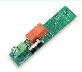
The WDA-600 combines with the RAK8-MB to provide a centralised lighting control system that can integrate with either wireless or wired Rako products.
