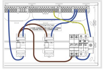
Fit the 6mm earth cable into one of the terminals in the top of the SPD and terminate in the earth bar. Torque to 3.6Nm.
