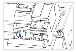
Loosen the bottom terminals on the Main switch and Surge protection device and insert the busbar into the rectangle slots above the cage terminals.
