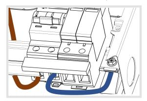
Push the busbar firmly against the Surge protection device making sure the cables below are secure secure and torque back to 3.6Nm.
