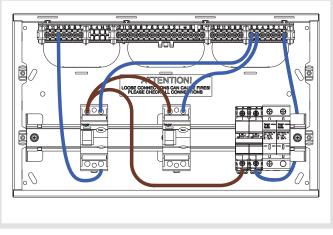
Move the main switch over 2 modules and clip the Surge protection device on the right hand side of the main switch.
