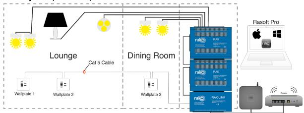
The RAK-LINK is used to integrate the RAK(s) into the Rako Wired Network and can support a total of 32 circuits. For example 4 RAK8s or 3 RAK8s and 2 RAK4s.
