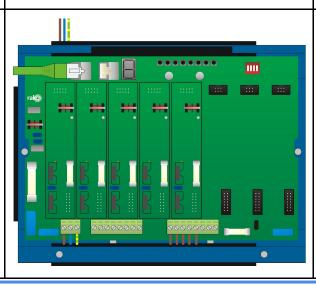
Insert the RJ45 cable from the RAK-LINK/RxLINK into the port on the RAK and from there another RJ45 cable to each RAK in the "stack".
