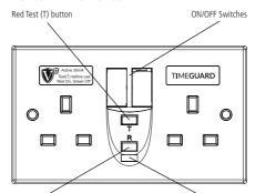
Blue Reset button (R) for RCD01WAVN, Status indicator shows Red Grey Reset button (R) for RCD02WPVN
