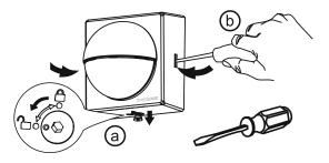
5.4 With both lugs pressed in, remove the font cover by pulling it away from the PIR sensor (See image 3).
