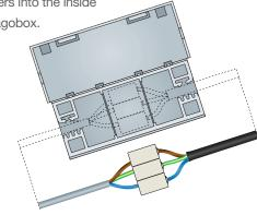
7 Push the cables down into the clamps as far as they will go. Close the lid and snap shut.
