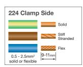
3 Connect the cables together to make the circuit
