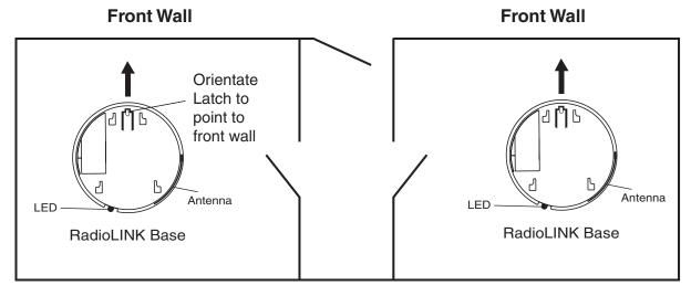
Orientate all RadioLINK bases in the same direction
