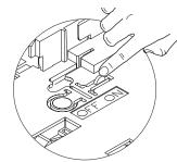
Press and hold the test button. The red led will flash and the horn will sound.
