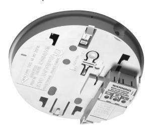
The primary function of the RadioLINK base is to interconnect all Alarms in the system, i.e. when one Alarm senses fire, the Ei168RC base attached to that Alarm will transmit an RF signal that will activate the sounders in all the other Alarms.
