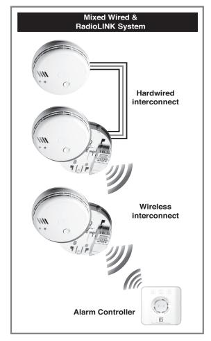
In this configuration the alarm controller must be a RadioLINK device. It is not possible to control the system from the hardware interconnect side
