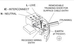
Slide the Alarm head onto the base. Connect the mains power to the alarm circuit.
